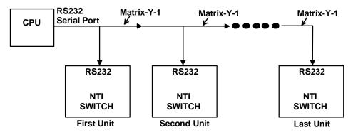
Figure 14- RS232 connection with Matrix-Y-1 cable
